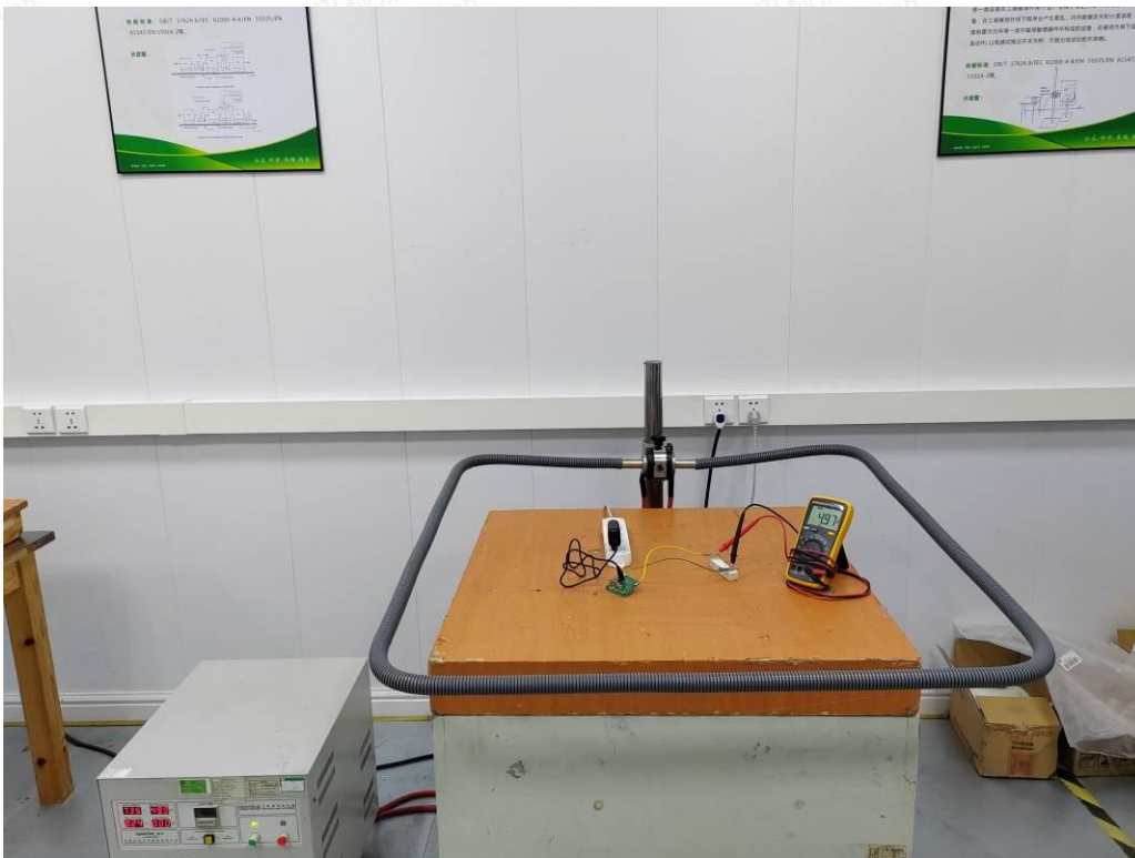
Test Setup Photo of Magnetic Field Susceptibility Test
