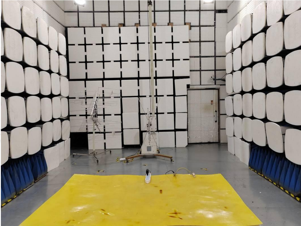
Test Setup Photo of Radiated Measurement (30MHz~1GHz)
