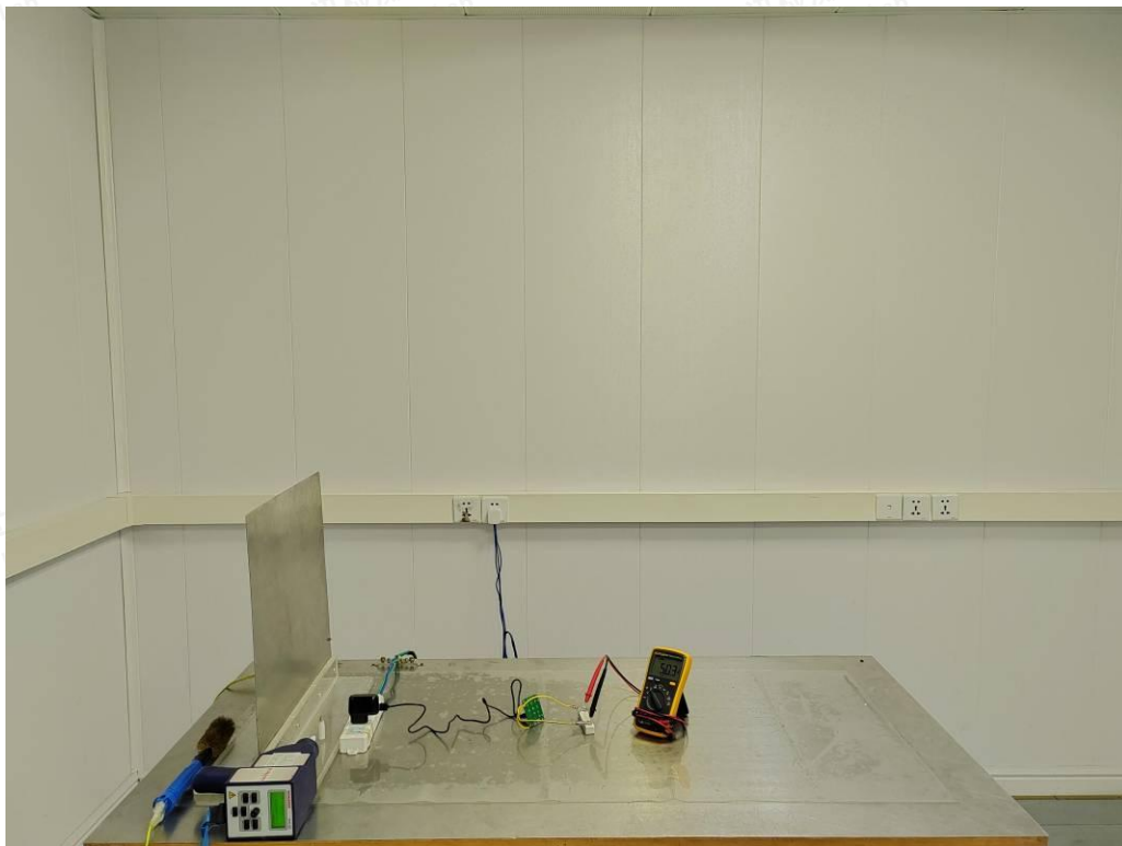
Test Setup Photo of Electrostatic Discharge Test
