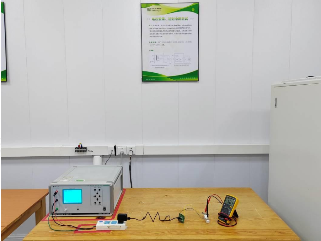
Test Setup Photo of Voltage Dips and Interruptions Test
