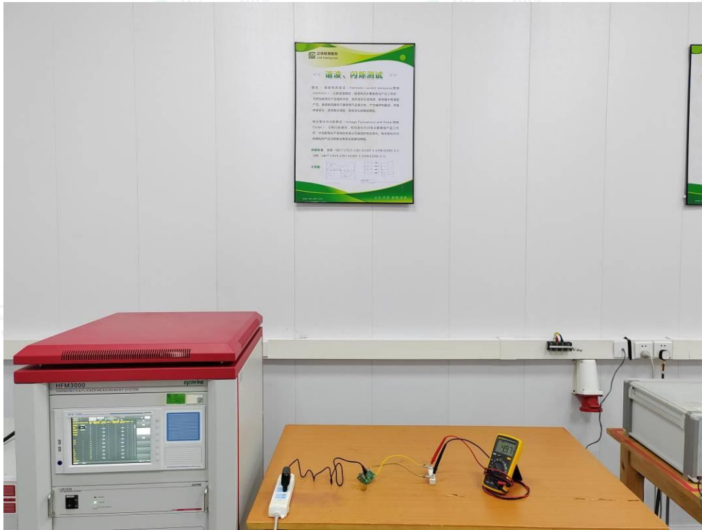
Test Setup Photo of Harmonic & Flicker Measurement
